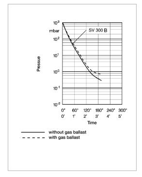
Pump-down characteristics of a 1000 I vessel at 50 Hz
