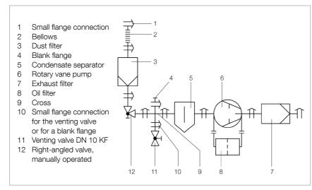
Example of connecting a pump with accessories
