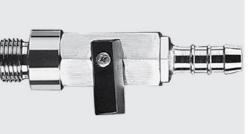
This oil drain tap may be screwed into the oil drain when wanting to change the oil in the rotary vane pumps. It is also suited for the condensate separators and exhaust filters of the TRIVAC B series.
