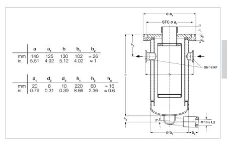
Dimensional drawing for the TK 4-8 cold trap
