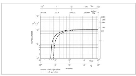
Pumping speed characteristics for the SOGEVAC SV 100 B at 60 Hz
