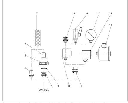
The fittings presented have been specially matched to the SOGEVAC pumps. We recommend to use only these or other components from Leybold for connecting SOGEVAC pumps, so as not to impair the pumping speed of the pumps or the leak tightness of the system.
