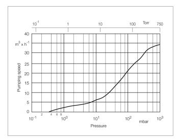
Pumping speed characteristics of the SOGEVAC SV 40 ATEX at 50 Hz for gases of the material group IIB + H<sub>2</sub> (60 Hz curves at the end of the chapter)
