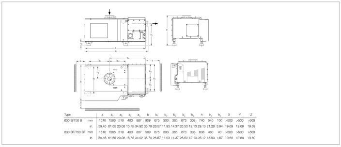
Dimensional drawing for the SOGEVAC SV 630 B, SV 630 BF, 750 B and 750 BF
