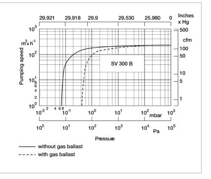
Pumping speed characteristics of the SOGEVAC SV 300 B at 50 Hz  $(60\ Hz\ curves\ at\ the\ end\ of\ the\ chapter)$
