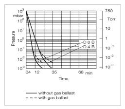
Pump-down characteristics of a 10 I vessel at 50 Hz
