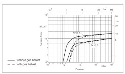
Pumping speed characteristics of the SOGEVAC SV 10 B and SV 16 B at 50 Hz (60 Hz curves at the end of the chapter)
