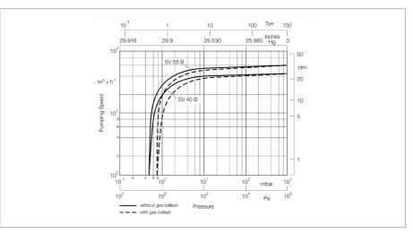
Pumping speed characteristics for the SOGEVAC SV 40 B and SV 65 B at 60 Hz
