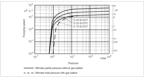
Pump-down characteristics of a 10 I vessel at 50 Hz Pumping speed characteristics at 50 Hz (60 Hz curves at the end of the chapter)
