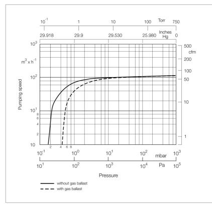
Pumping speed characteristics of the SOGEVAC SV 120 B at 50 Hz (60 Hz curves at the end of the chapter)
