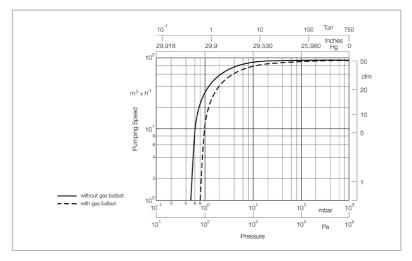
Pumping speed characteristics of the SOGEVAC SV 100 B at 50 Hz (60 Hz curves at the end of the chapter)
