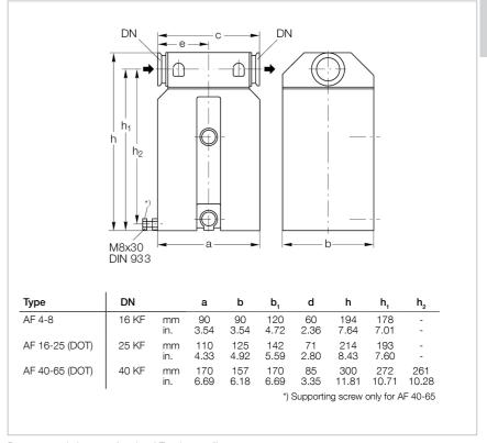
Dimensional drawing for the AF exhaust filters
