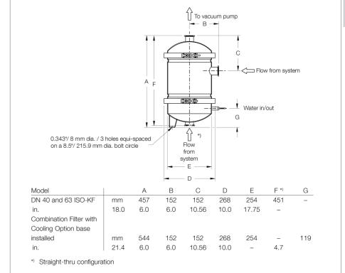
Dimensional drawing for the combination filter
