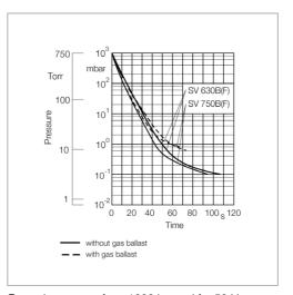
Pumpdown curve for a 1000 I vessel for 50 Hz pump operation
