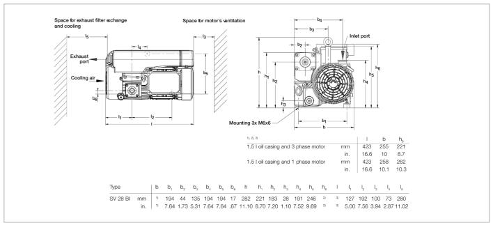
Dimensional drawing for the SOGEVAC SV 28 BI with standard single-phase motor, European version (dimensions for three-phase motor smaller)
