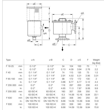
Dimensional drawing for the dust filters F 16-25 to F 630
