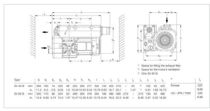
Dimensional drawing for the SOGEVAC SV 40 B and SV 65 B with standard motor, European version
