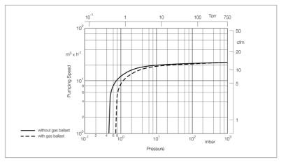
Pumping speed characteristics of the SOGEVAC SV 25 B at 50 Hz
