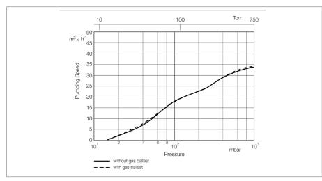
Pumping speed characteristics of the SOGEVAC SV 40 ATEX at 60 Hz for gases of the material group IIB and H<sub>2</sub>
