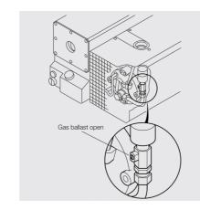
The pumps SOGEVAC SV 10 B, SV 16 B and SV 25 B are equipped depending of their Part No. without or with a permanent gas ballast.
