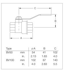
Dimensional drawing for the ball valves BV
