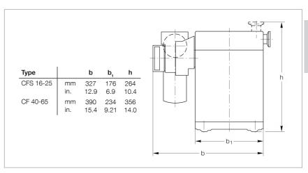
Dimensional drawing for the CFS (mounted on a TRIVAC BCS)
