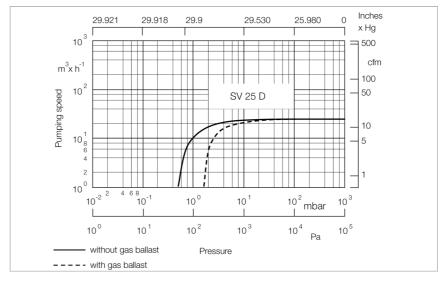
Pumping speed characteristics of the SOGEVAC SV 25 D at 50  $\mbox{Hz}^{\star}$
