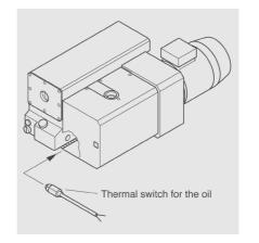
The thermal switch is installed at the hottest point of the pump module. It responds as soon as the temperature of the pump exceeds the maximum operating temperature. This accessory is recommended when operating the pump at high ambient temperatures.
