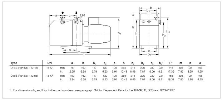
Dimensional drawing for the TRIVAC D 4 B and D 8 B
