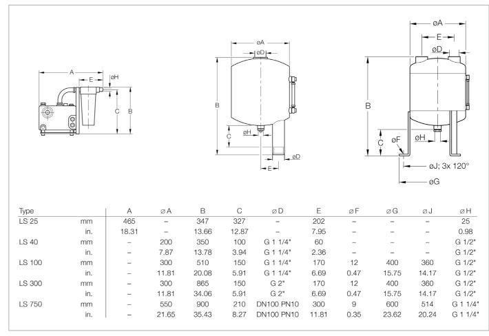
Dimensional drawings for the separators; LS 25 (left), LS 40 (middle) and LS 100 up to LS 750 (right)
