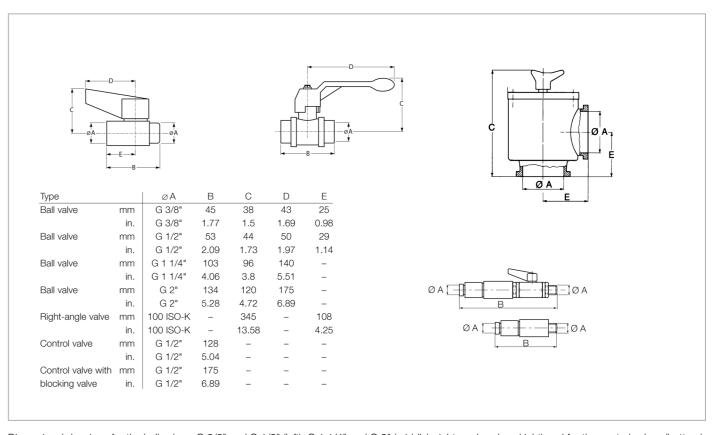
$Dimensional \ drawings \ for \ the \ ball \ valves; \ G\ 3/8" \ and \ G\ 1/2" \ (left), \ G\ 1\ 1/4" \ and \ G\ 2" \ (middle), \ right-angle \ valves \ (right) \ and \ for \ the \ control \ valves \ (bottom)$
