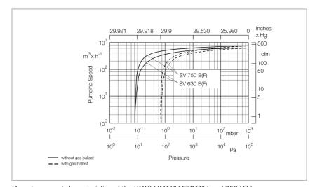
Pumping speed characteristics of the SOGEVAC SV 630 B(F) and 750 B(F) (60 Hz curves at the end of the chapter)
