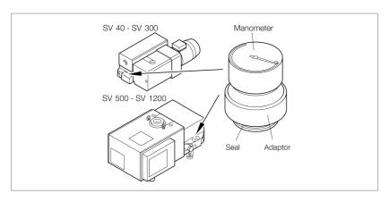
The manometer (40 mm (1.58 in.) dia.), glued in the adapter, is installed instead of the oil filling plug. Dial has 2 colors:
