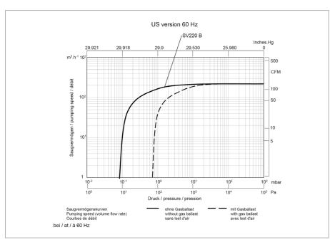
Pumping speed characteristics for the SOGEVAC SV 220 B at 60 Hz
