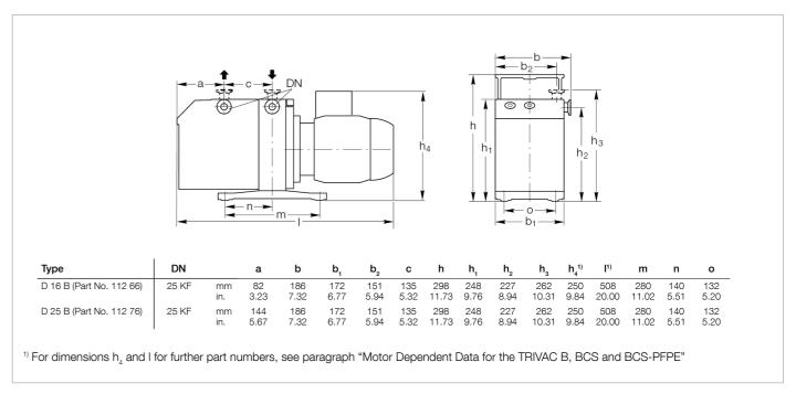
Dimensional drawing for the TRIVAC D 16 and D 25 B
