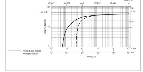
Pumping speed characteristics of the SOGEVAC SV 40 BI at 50 Hz (60 Hz curves at the end of the chapter)
