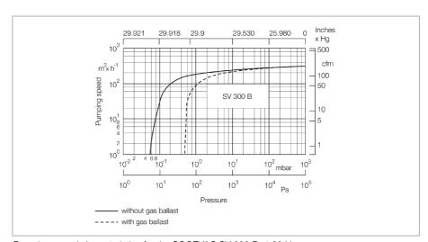
Pumping speed characteristics for the SOGEVAC SV 300 B at 60 Hz  $\,$
