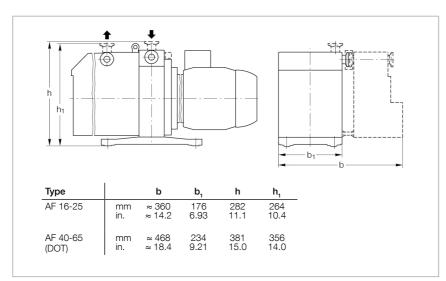
Dimensional drawing for the ARS mounted on a TRIVAC BCS
