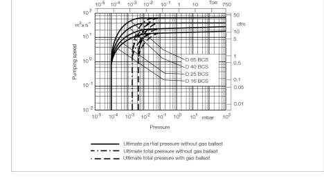
Pump-down characteristics of a 100 I vessel at 50 Hz
