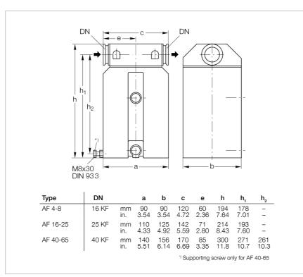
Dimensional drawing for the AK condensate separators
