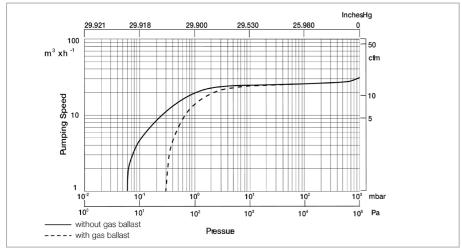
Pumping speed characteristics for the SOGEVAC SV 28 Bl at 60 Hz
