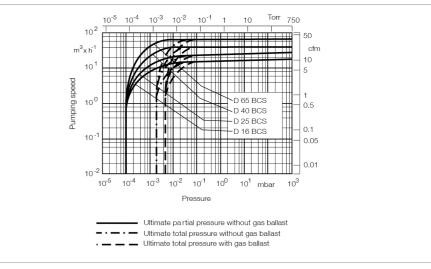
Pumping speed characteristics at 50 Hz (60 Hz curves at the end of the chapter)
