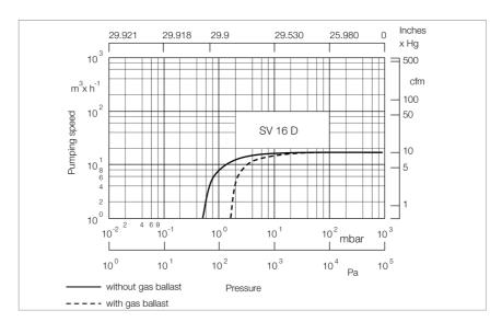
Pumping speed characteristics of the SOGEVAC SV 16 D at 50  $\mathrm{Hz}^{\star}$
