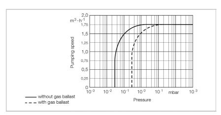
Pumping speed characteristics at 50 Hz
