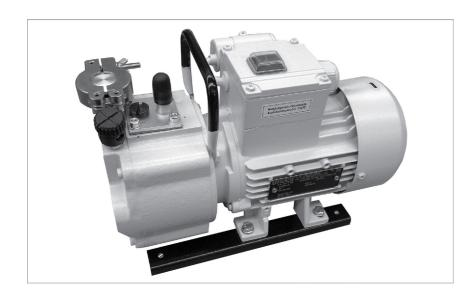
The S 1,5 is a single-stage, oil sealed rotary vane pump with a gas ballast valve. It is driven by a flange mounted AC motor. The shaft of the pump and the shaft of the motor are linked by means of a pinned coupling.
