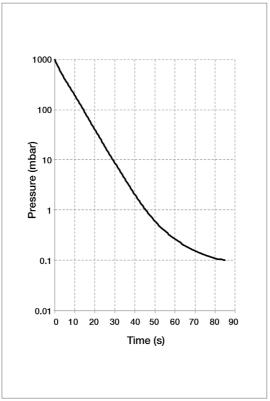
Pump-down characteristics of a 300 I vessel at 50 Hz
