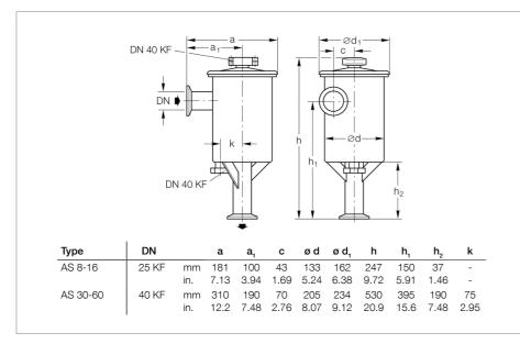
Dimensional drawing for the AS dust separators
