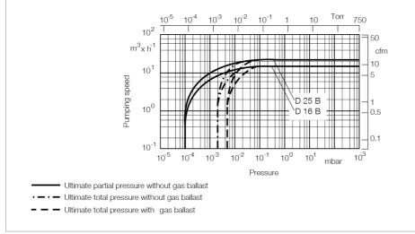
Pump-down characteristics of a 100 I vessel at 50 Hz Pumping speed characteristics at 50 Hz (60 Hz curves at the end of the chapter)
