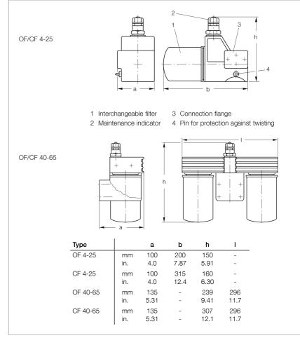
Dimensional drawings for the OF mechanical oil filters and CF chemical oil filters
