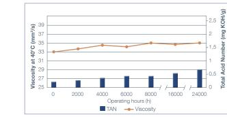
**LVO 700** has a stable performance up to 24,000 hours thanks to its specific additives, which extend the wear parts and oil lifetime and prevent physical pump damage by keeping the TAN and viscosity level under control and stable.
