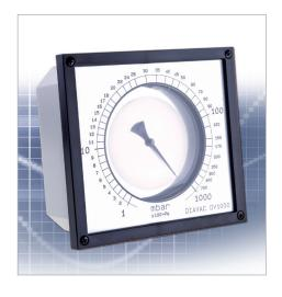
DIAVAC vacuum gauges are used for pressure measurements in the rough vacuum range from 1000 to 1 mbar. The DIAVAC DV 1000 is a rugged **mechanical** diaphragm vacuum gauge with high measurement accuracy.
