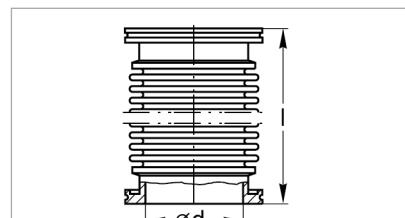
Dimensional drawing for the flexible vacuum hoses
