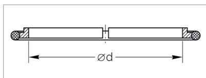
Dimensional drawing for the copper gaskets
