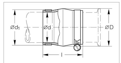
Dimensional drawing for the compensation elements with integrated support ring
