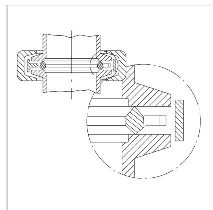
Small flange connection with ultra sealing ring
