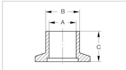
Dimensional drawing for the ISO-KF flanges with weld stub
