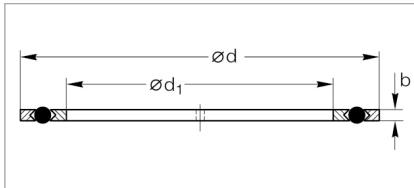
Dimensional drawing for vacuum sealing disks
