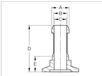
Dimensional drawing for the ISO-KF nipples
