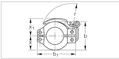
Dimensional drawing for the quick clamping rings
