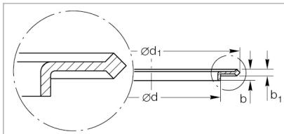
Dimensional drawing for the ultra sealing disks
