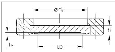
Dimensional drawing for the CF blank flanges,
