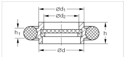
Dimensional drawing for the centering rings with O-ring
