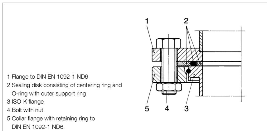
Connection between a DIN EN 1092-1 ND 6 flange and an ISO-K flange with DIN EN 1092-1 collar flange
