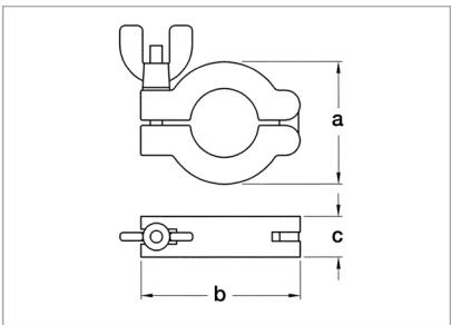
Max. torque at the wing nut: 2 Nm
