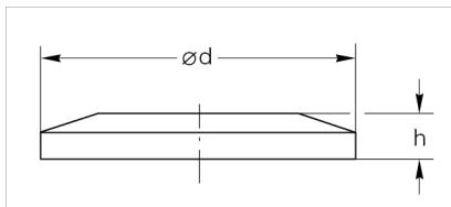
Dimensional drawing for the outer support rings
