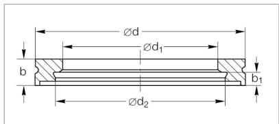
Dimensional drawing for the welding flanges
