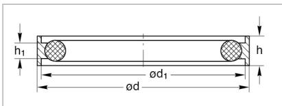
Dimensional drawing for the outer centering rings with O-ring
