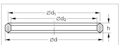
Dimensional drawing for the ultra sealing rings
