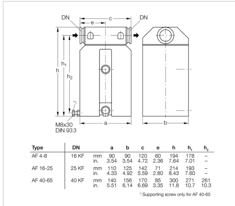
Dimensional drawing for the AK condensate separators
