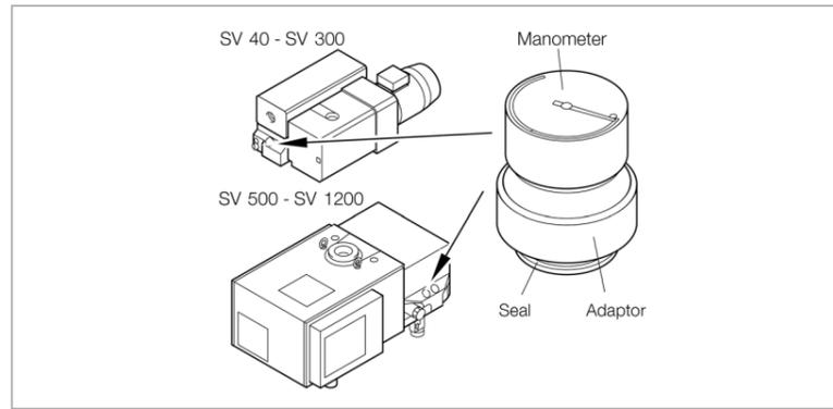
The manometer (40 mm (1.58 in.) dia.), glued in the adapter, is installed instead of the oil filling plug. Dial has 2 colors:
