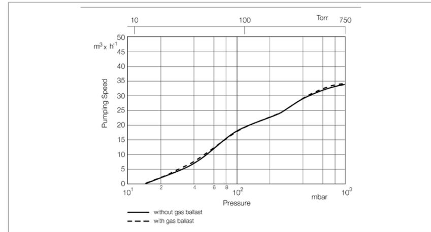
Pumping speed characteristics of the SOGEVAC SV 40 ATEX at 60 Hz for gases of the material group IIB and H<sub>2</sub>
