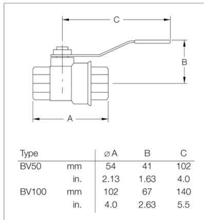
Dimensional drawing for the ball valves BV
