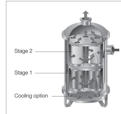
Combination filter: cutaway view
