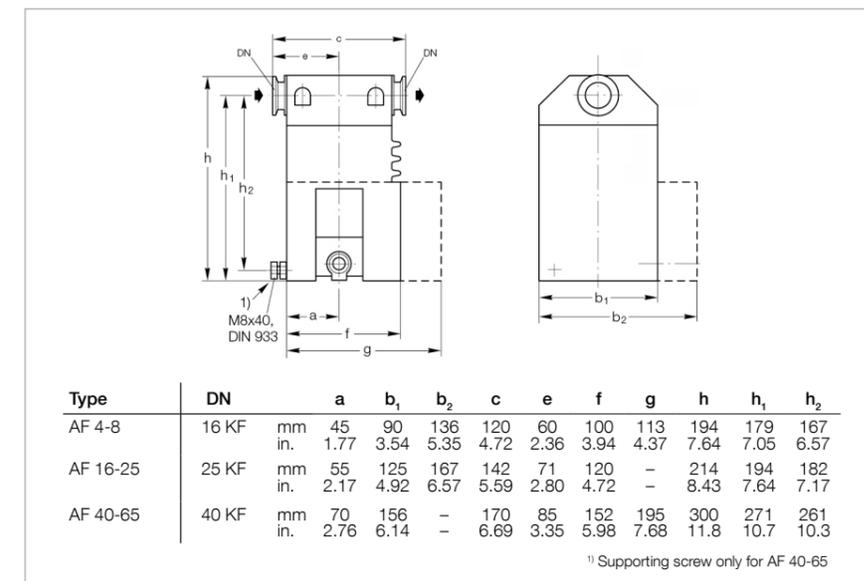
Dimensional drawing for the AR exhaust filters with lubricant return (dimensions for the ARP exhaust filter with lubricant return upon request)
