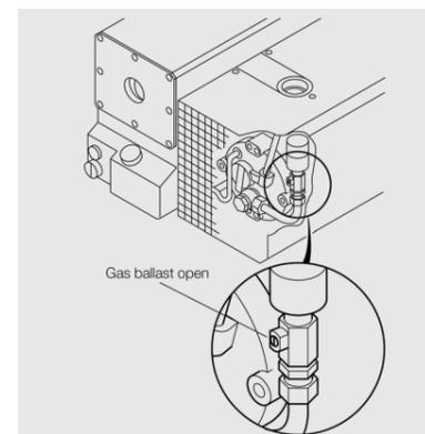
The pumps SOGEVAC SV 10 B, SV 16 B and SV 25 B are equipped depending of their Part No. without or with a permanent gas ballast.
