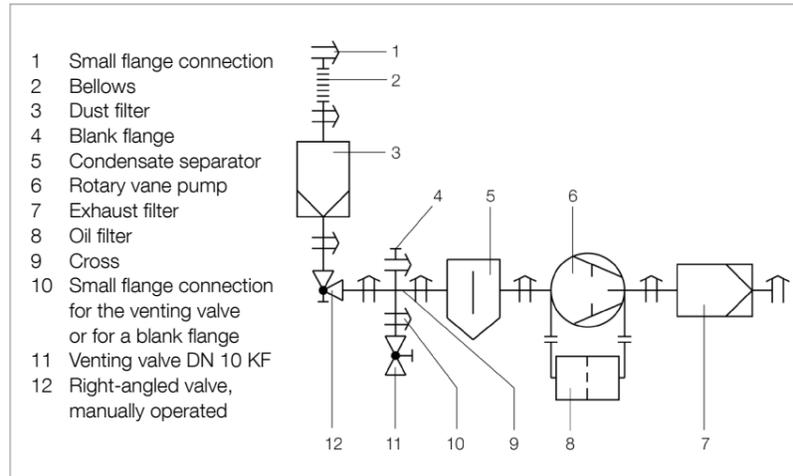
Example of connecting a pump with accessories
