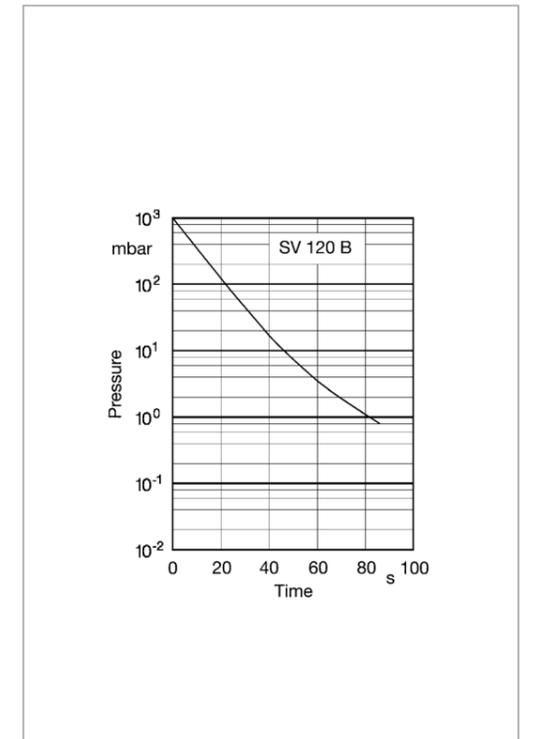
Pump-down characteristics of a 300 l vessel at 50 Hz
