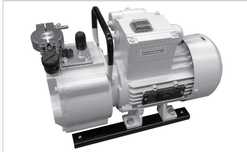
The S 1,5 is a single-stage, oil sealed rotary vane pump with a gas ballast valve. It is driven by a flange mounted AC motor. The shaft of the pump and the shaft of the motor are linked by means of a pinned coupling.
