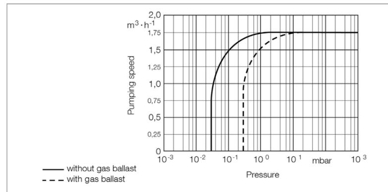
Pumping speed characteristics at 50 Hz
