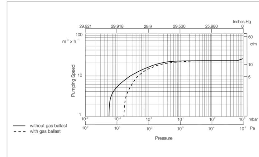
Pumping speed characteristics of the SOGEVAC SV 28 BI at 50 Hz
