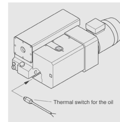
The thermal switch is installed at the hottest point of the pump module. It responds as soon as the temperature of the pump exceeds the maximum operating temperature. This accessory is recommended when operating the pump at high ambient temperatures.
