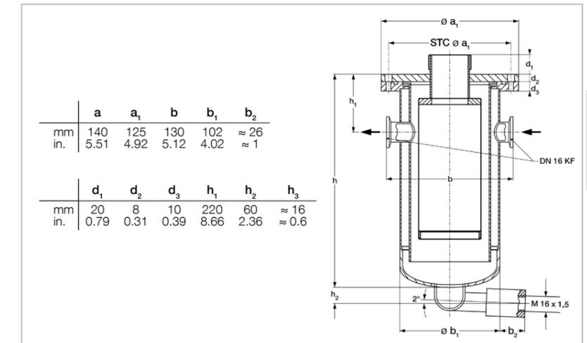
Dimensional drawing for the TK 4-8 cold trap
