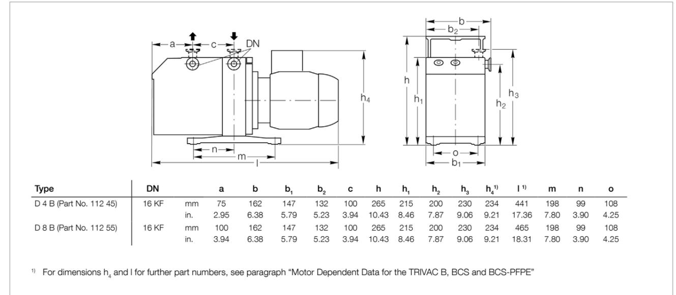
Dimensional drawing for the TRIVAC D 4 B and D 8 B
