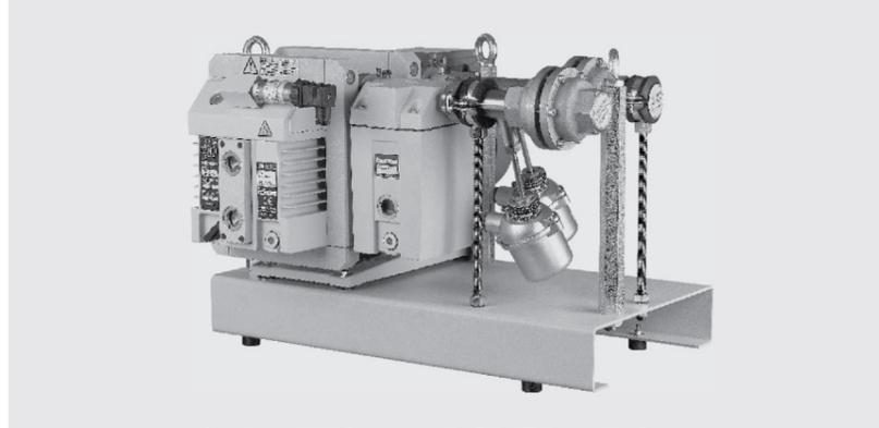
Vacuum pumps TRIVAC D 16 B-Ex meet the requirements of the European Directive 2014/34/EU (ATEX Directive). TRIVAC D 16 B-Ex pumps are classified inside as Category 1, outside as Category 2. Thus these pumps are suited for pumping explosive gases from Zone 0, the pump itself may be located in Zone 1.
