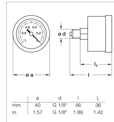
Dimensional drawing for the Bourdon vacuum gauge Part No. 951 90
