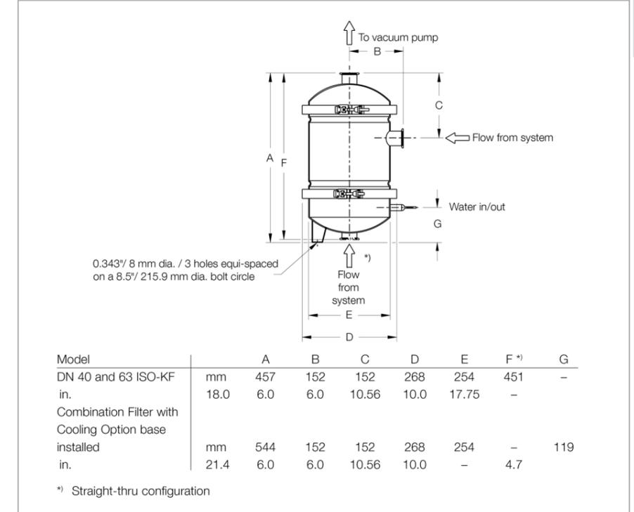
Dimensional drawing for the combination filter
