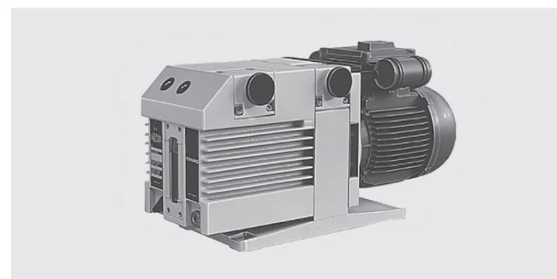
The TRIVAC B-DOT pumps operate with brake fluid (DOT 4) as the sealing and lubricating agent. Therefore these pumps are equipped with EPDM seals. EPDM is highly compatible with brake fluid.
