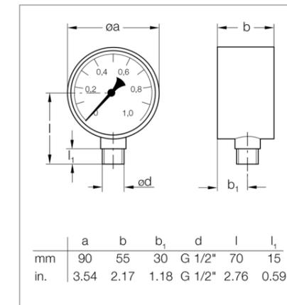
Dimensional drawing for the Bourdon vacuum gauge Part No. 951 92
