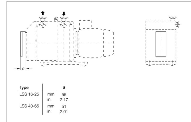
Dimensional drawing for the LSS (mounted on a TRIVAC BCS)
