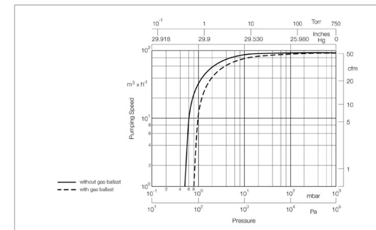
Pumping speed characteristics of the SOGEVAC SV 100 B at 50 Hz
