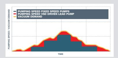
Multi-VAControl™ manages the load between the connected pumps to ensure that your pumps run at the minimum required level.
