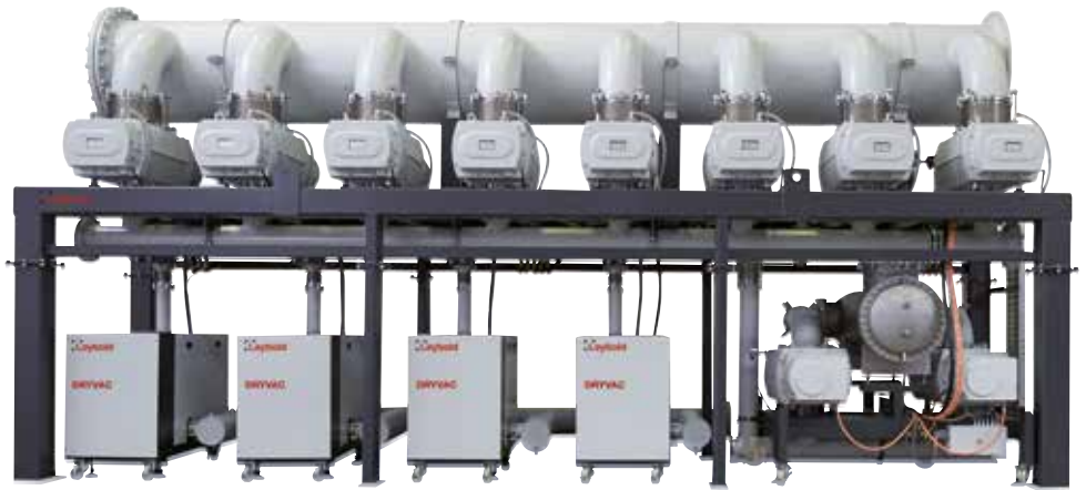
Custom-made, ATEX-compliant steel degassing system comprising DRYVAC 1200 and RUVAC WH 7000
