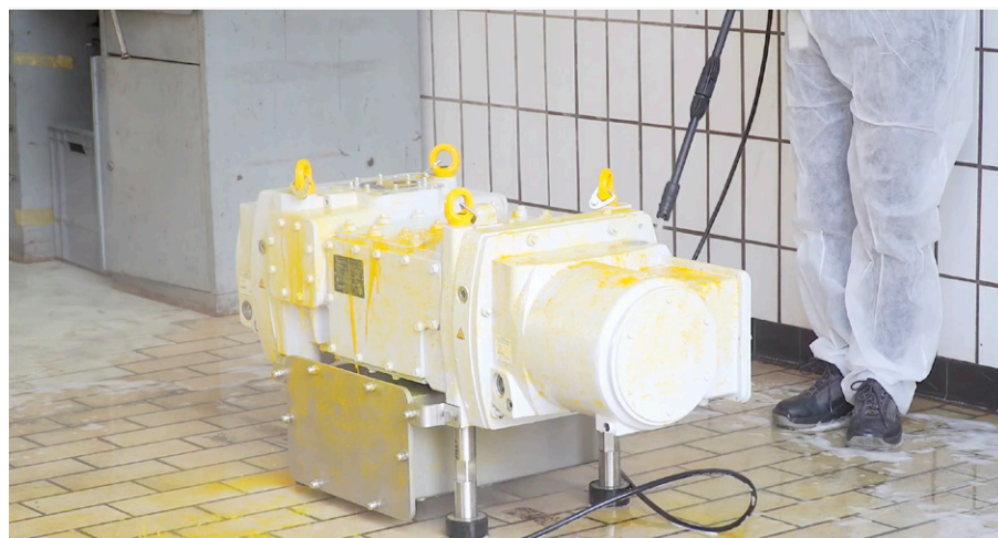
DRYVAC DV 650 FP-r designed for wash-down environment
