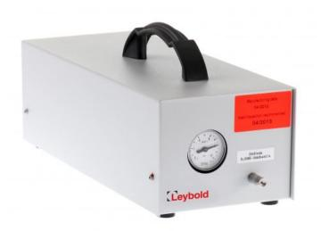
In the so-called sniffer technique, another variation of the of the positive pressure technique, the (test) gas issuing from leaks is collected (extracted) by a special apparatus and fed to the leak detector. This procedure can be carried out using either helium, refrigerants, SF6 as the test gas.
