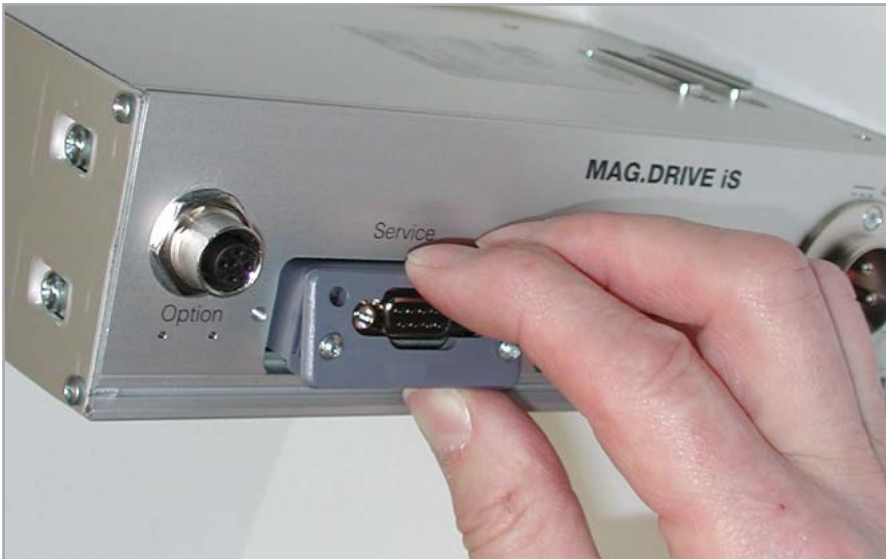
Fig.2.3 Inserting the module
