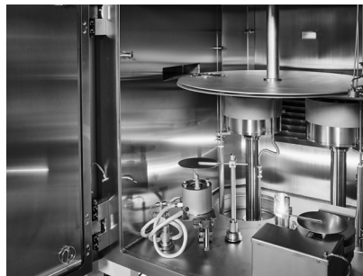
Chamber bottom: In the front, an ion source and an electron beam evaporator with multiple rotating crucible. In the rear, two magnetron sputter sources.
