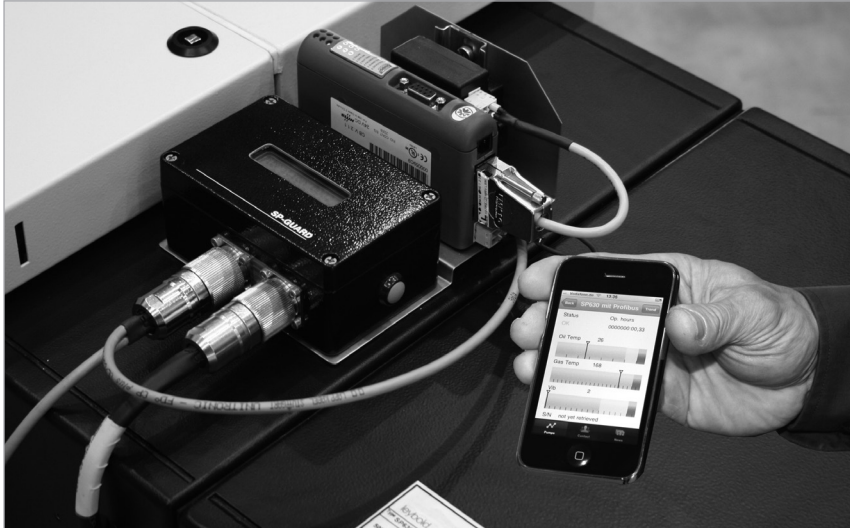
Wi-Fi and Profibus interface kit for SP-GUARD
