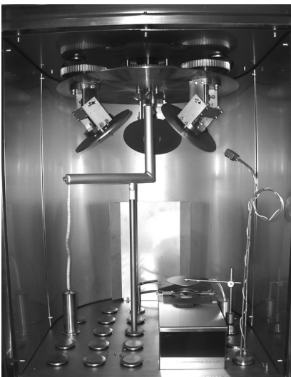
Chamber bottom: electron beam evaporator with sixfold rotating crucible
